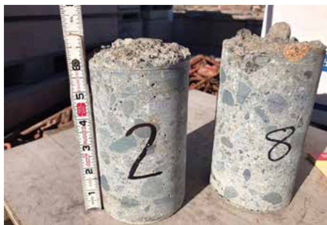
Fig. 10: A view of the irregular bottom surfaces of Cores 2 and 8. The range of nine measurements on these two cores were the highest, with Core 2 at 0.25 in. and Core 8 at 0.375 in. This range indicates the measuring issue for concrete cores removed from an open-graded aggregate base
